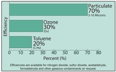
Camfil's unique molecular filtration testing laboratory runs tests according to the following standards: ASHRAE 145.1, ASHRAE 145.2, ISO 10121-1 and ISO 10121-2. The initial removal efficiencies referenced in the chart above were determined by challenging full size (24" x 24") filters with realistic gas concentrations in 2,000 CFM of air at 50% RH and 72F. More information on this unique testing facility can be provided.
