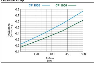
(Schedule air filters for change when initial pressure drop has doubled.) Final pressure drop should not exceed 1.2" w.g.
